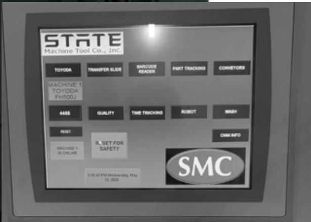
The cell's main HMI screen allows the operator to track the machining of parts and all safety functions (operator access doors).
