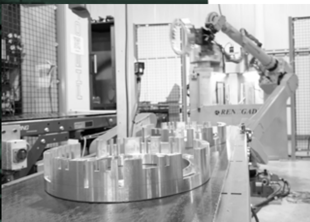
Parts leaving the lathe on the way to the robot which places them in the mill (left) and then the washer/dryer (behind the robot).
